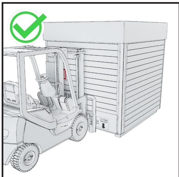
Drive forklift under the module from front.
