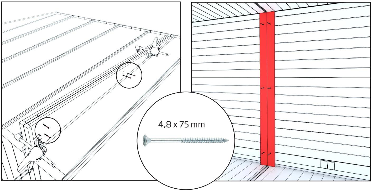
**4. Attach the lounge XL modules together from the roof side using four screws.**
