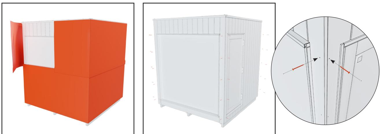
9. Remove the white packaging protection. Put the brown screws, with which the corner sheet metals were attached, back into the corner panels.
