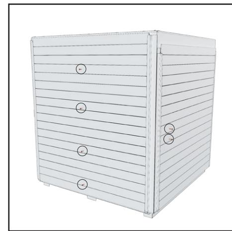
4. Remove the signs from the packaking. Remove all screws from the boards. These screws keep the supports inside the boards in place.
