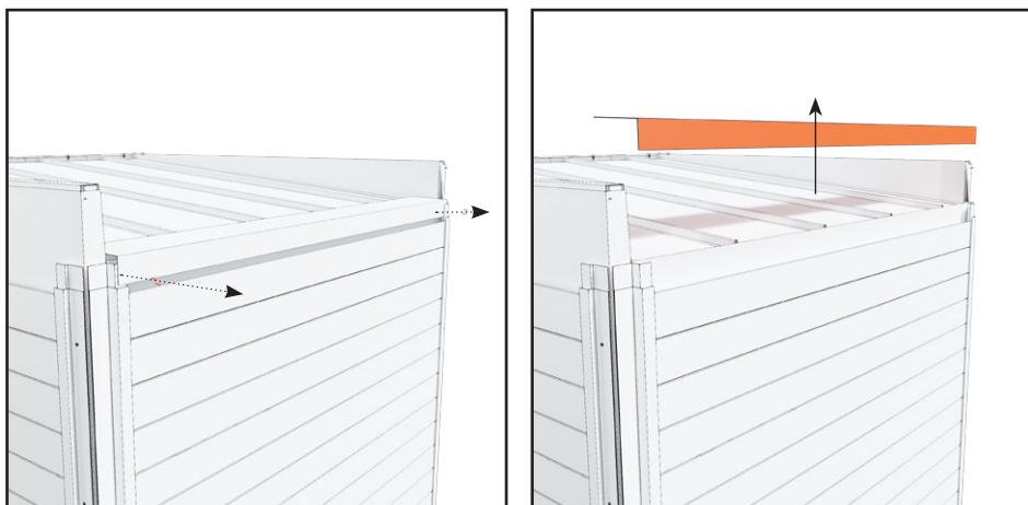
3. Remove the sheet metal from the rear edge of the roof. It is attached with two screws on both ends.
