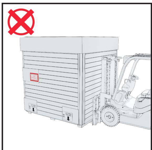
Do not ever drive the forklift from the side. This will result in damage of the module.
