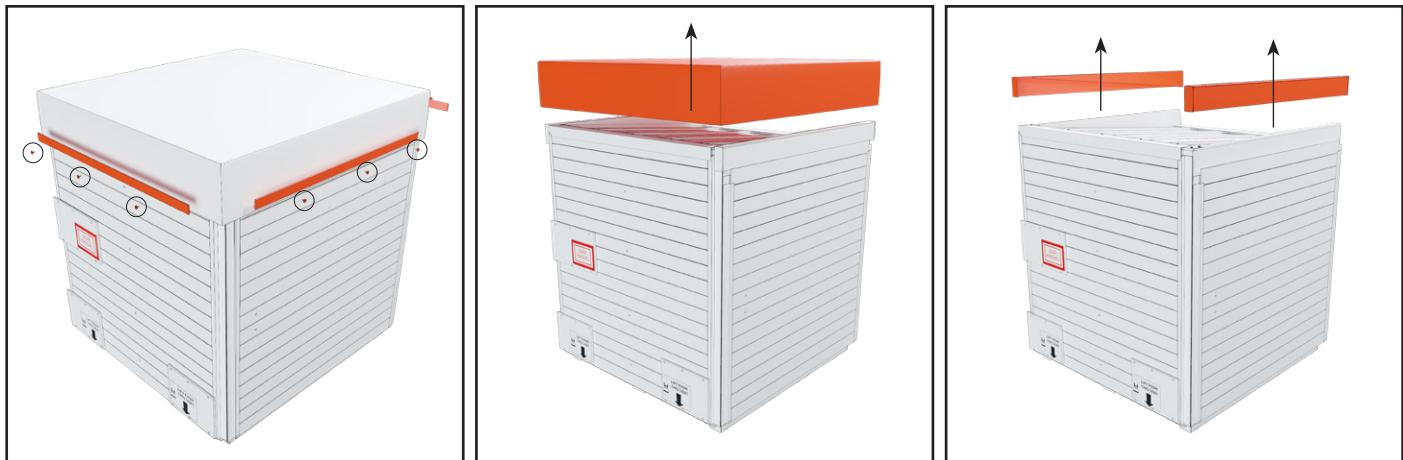
1. Remove the roof hood screws and lift the hood off. Lift the plywood boxes off the roof.
