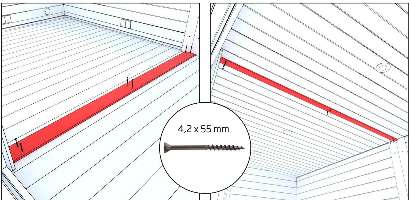
7. Place the cover strip on the floor between the modules and fasten with six screws. The strip has pre-drilled holes.
