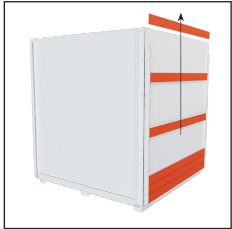
5. Boarding removal. A few upper boards (4-6) have to be lifted straight up and removed. The rest can be removed diagonally.
