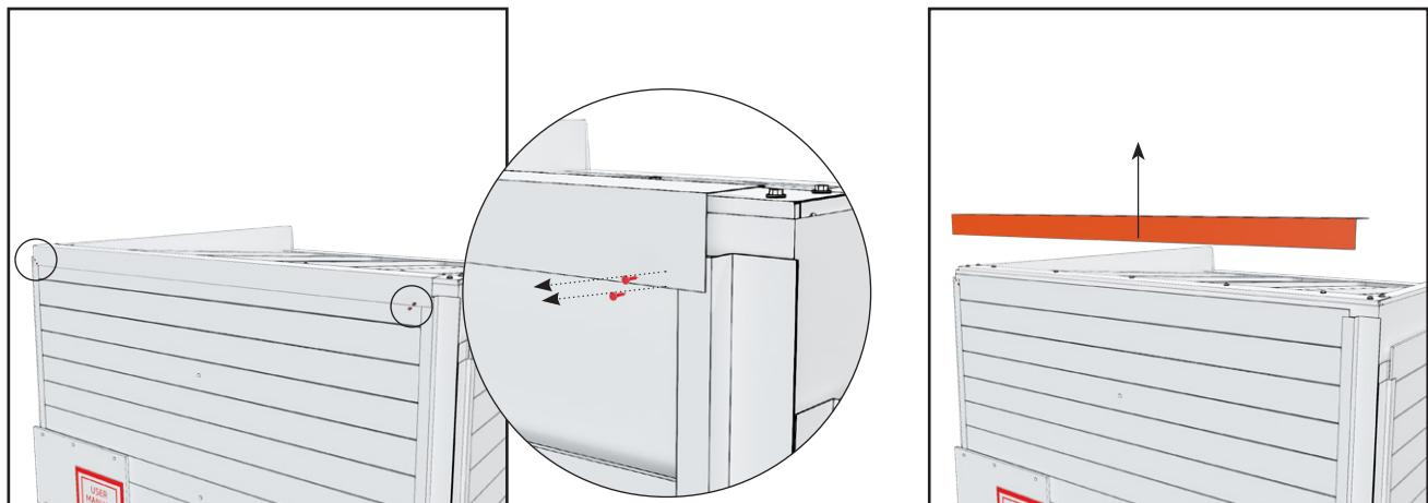
2. Remove the sheet metal from the front edge of the roof. It is attached with two screws on both ends.
