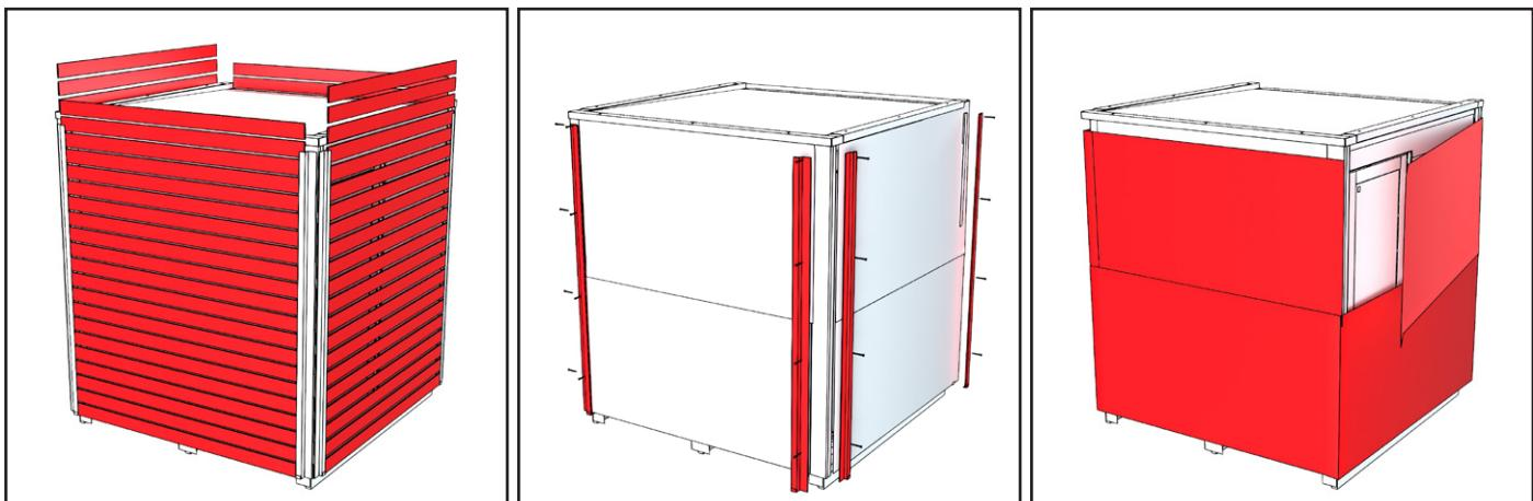
Lift off the protective boards and detach the corner metal sheets (8 pcs) from the edges of the sauna. Remove the white packaging protection around the sauna.
