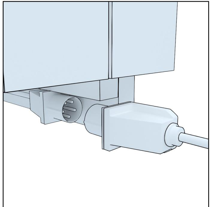
2. Connect the main power to the sauna. The connection can be found behind the sauna on the heater side.
