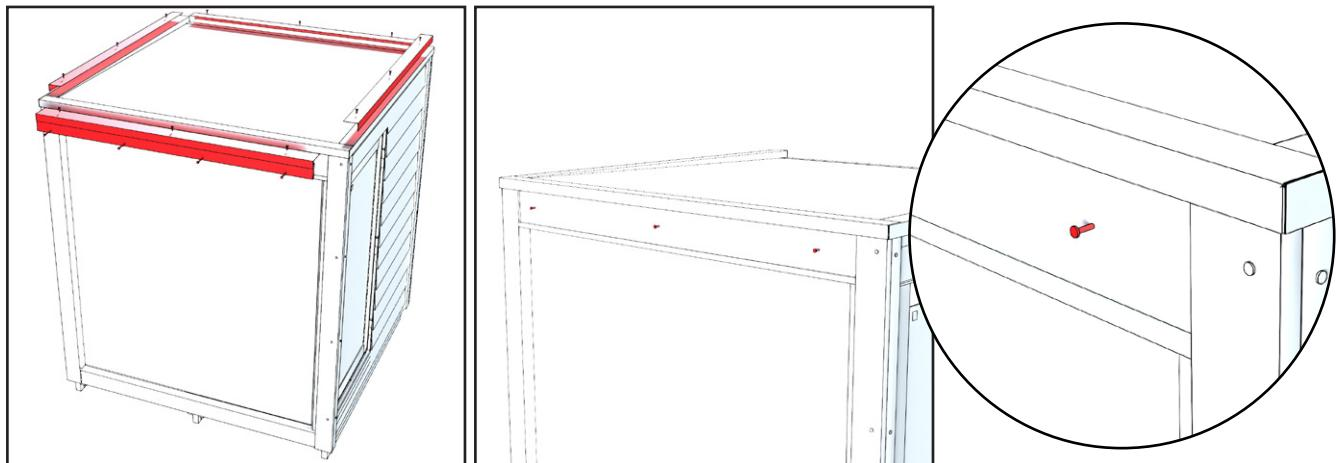
Remove the L-profile metal sheets on the sauna roof. The sheets are attached with screws from the top and to the board at the front of the sauna. Put the screws back in the front wall in the same spots where the cover was removed.
