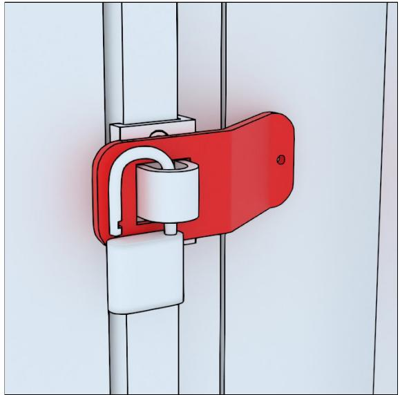
The door must be locked when not in use. This prevents the door from opening and breaking, eg in stormy weather
