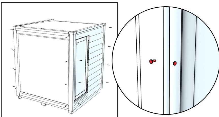
Put the screws that were used to attach the corner metal sheets back into the corner strips.
