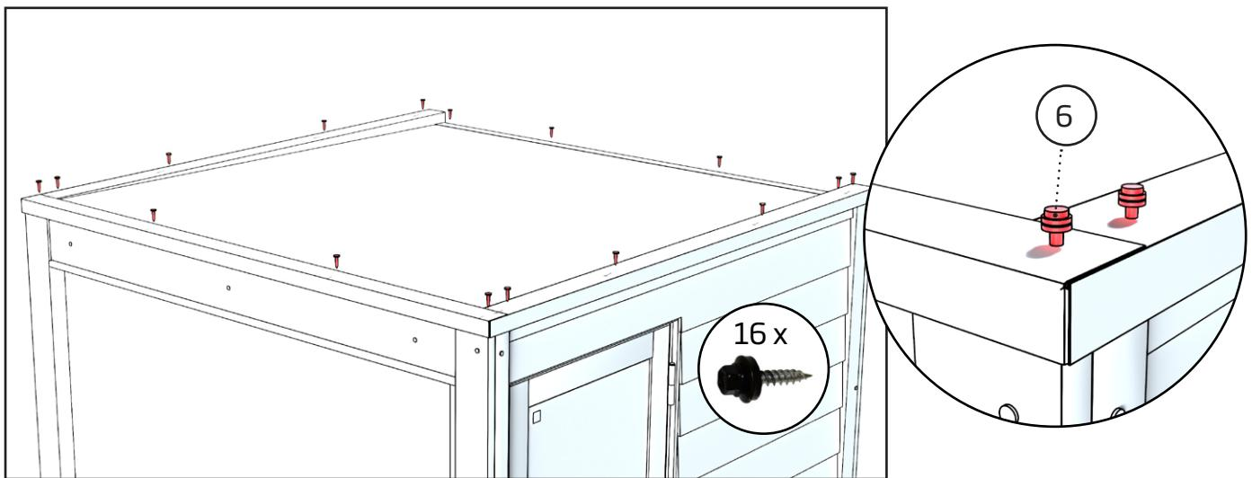
Fasten the edges of the roof sheet with new roofing screws. A total of 16 pieces.
