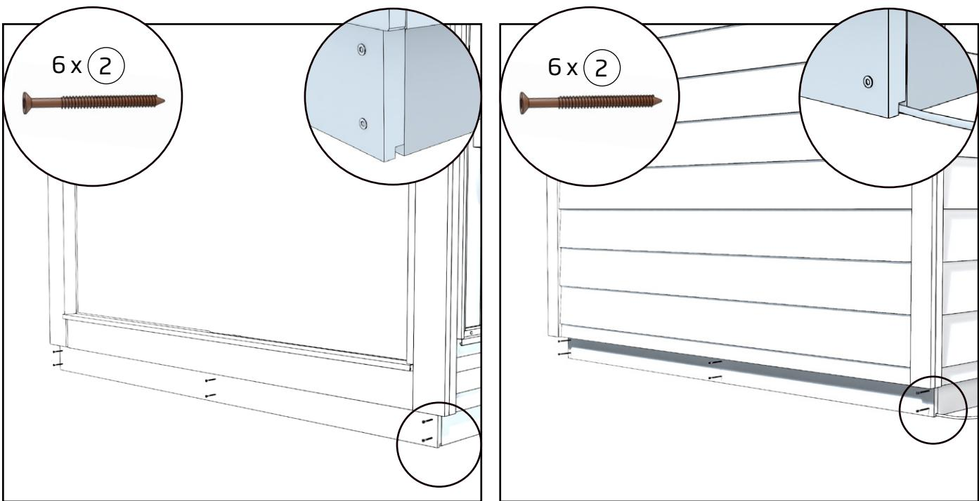
3. Install the cover strips on the transport supports at the front and rear with the 6 brown terrace screws.
