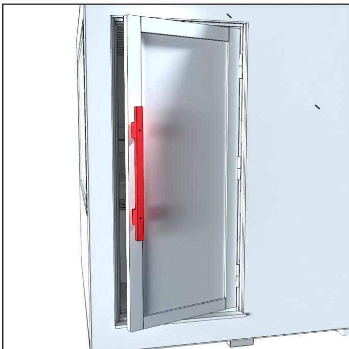
Attach the handle with two screws to the door.
