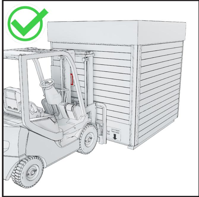
Drive forklift under the module from front.
