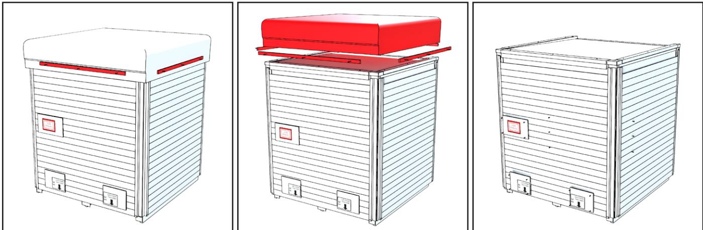
Remove the protective cover strips around the sauna and lift off the protective bag. Detach the signs and screws from the protective boarding.
