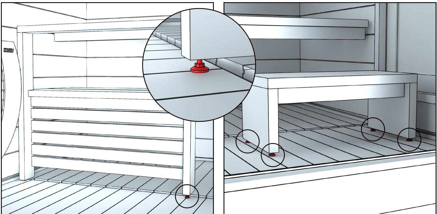
Tighten the railing's adjustable foot firmly against the floor. On the wall side of the edge, the adjustable foot is already set tight. Adjust the adjustment feet of the stool according to the floor slope to make them straight.
